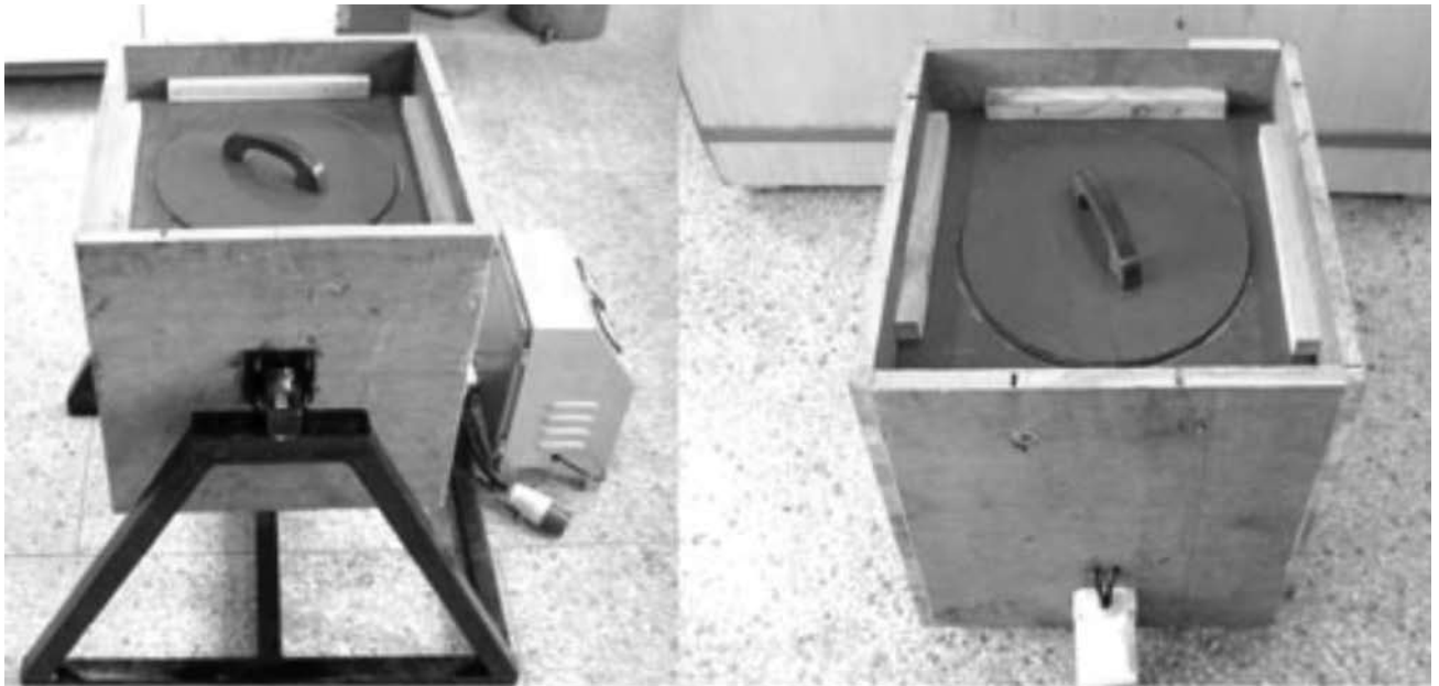
Fig. 1 Ohmic heating system enclosed in wooden frame (left) and mounted on a stand (right)
